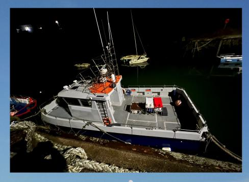
Constructed from GRP. Dimensions are length - 11m, beam - 5m and draught - 1.2m. The flush working deck area is a massive 50m squared with transom door and diving ladder to port. Spacious, heated wheelhouse with seating, PC equipment table (with 240v sockets) a navigation table cooking facilities & sink. Separate heads, below deck single berth and ample storage.
